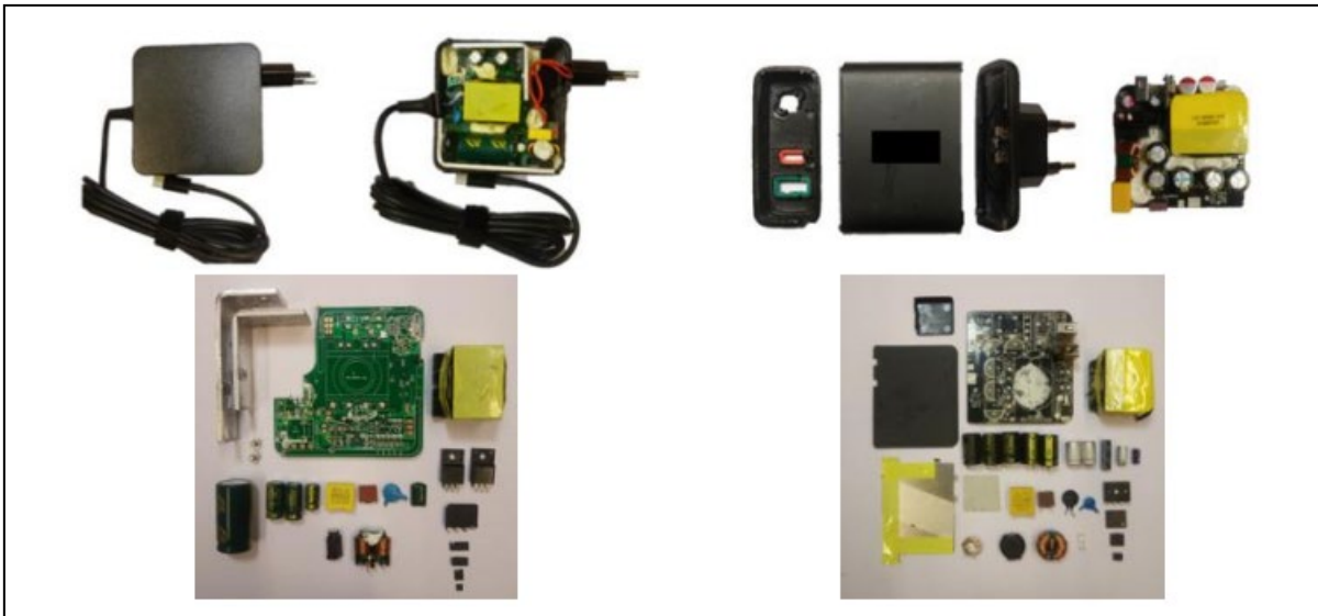
Figure 3 Laptop chargers investigated, on the left a 60W Si-based charger (reference), and on the right a 60W GaN-based charger.
