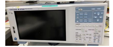
7 channel WT5000 Measuring electrical properties
